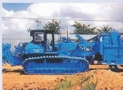
stabiliser Mixes the ground up to 50cm from the surface
